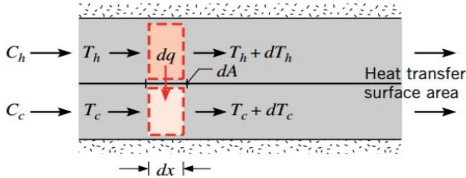
$$\ln\left(\frac{\Delta T_2}{\Delta T_1}\right) = -\frac{UA}{q} \left( (T_{q,e} - T_{f,e}) - (T_{q,s} - T_{f,s}) \right)$$
