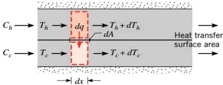
$$dq = -\dot{m}_q c_{p,q} dT_q = -C_q dT_q$$
